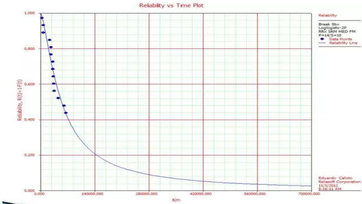
Figure 11 – Reliability function CDF example. Calixto Eduardo, Book RAMS and LCC Engineering for Railway Industry: Analysis, Modelling and Optimization.
