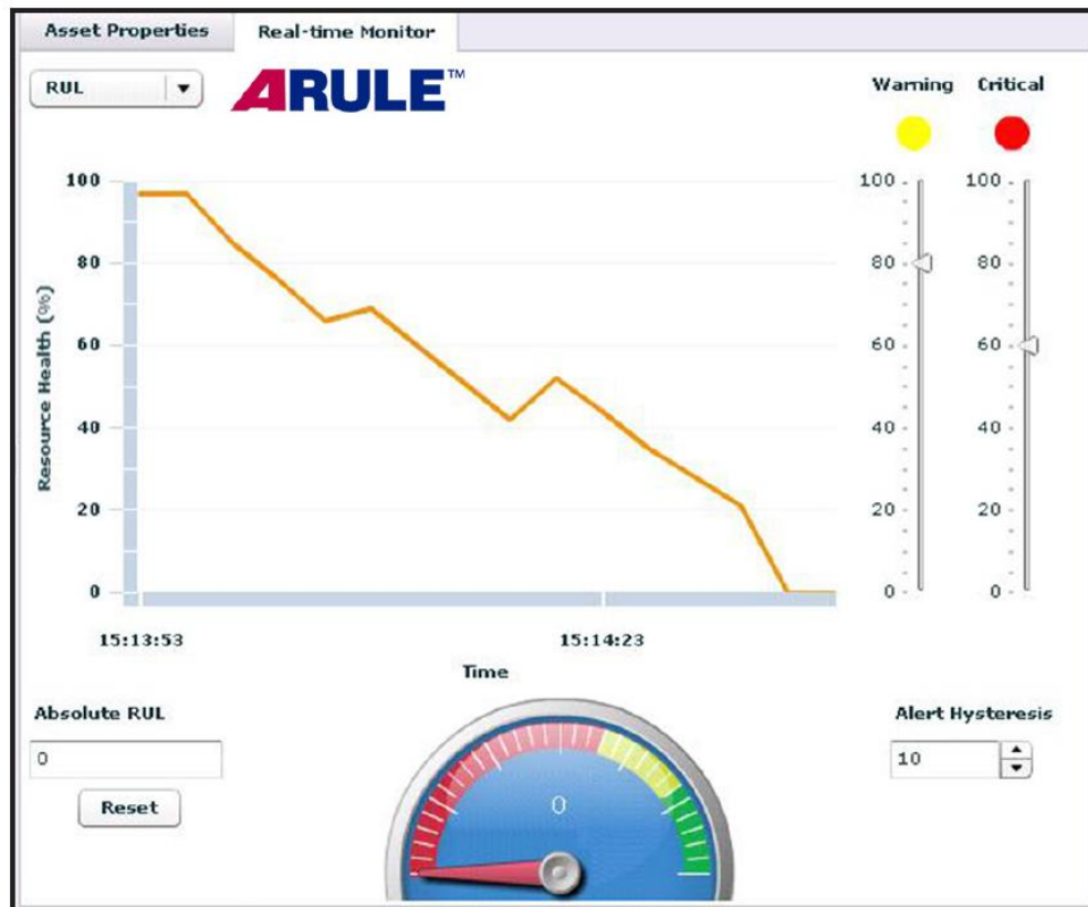
Remaining useful life representation of a system with ARULE API deployed in a Sentinel IT™ application
