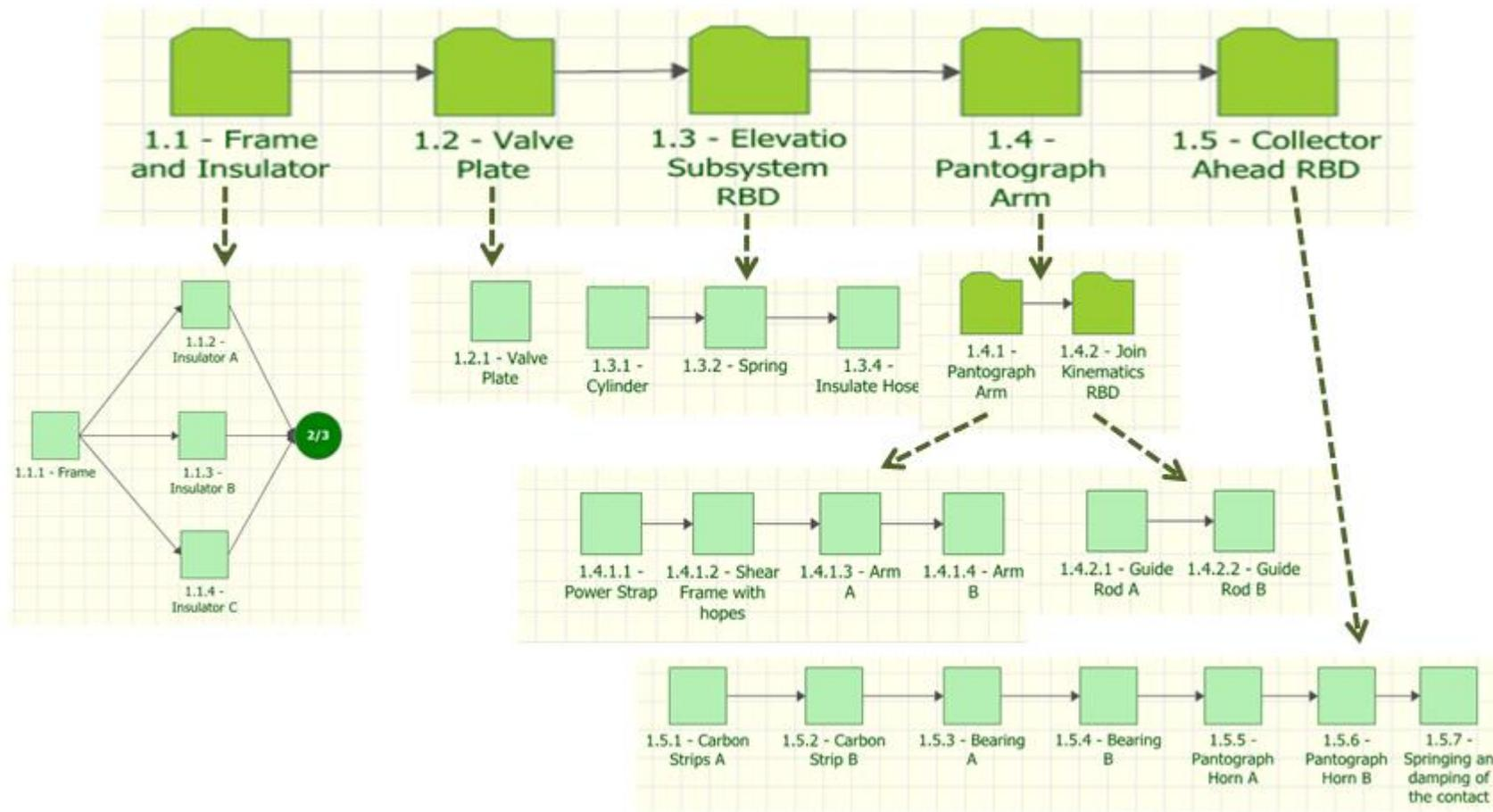
Figure 6 Pantograph RBD (Top Down configuration)
