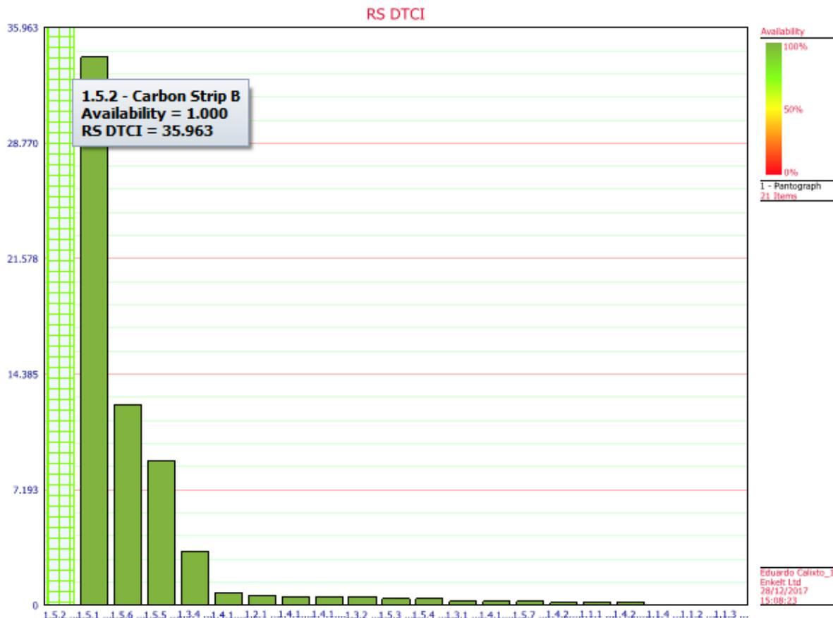
**Figure 9 Pantograph criticality analysis (DTCl 20 years)**
