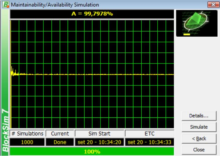
**Figure 4 Monte Carlo Simulation (Reliasoft Blocksim Software)**
