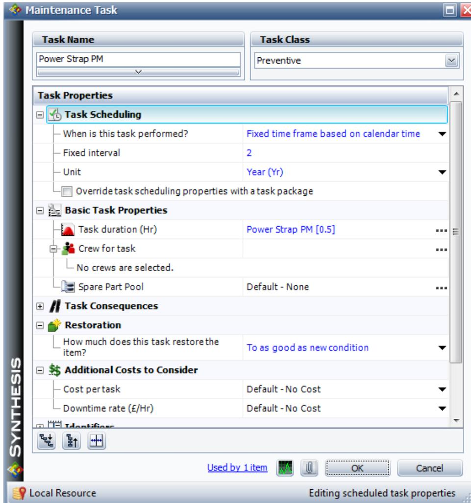
**Figure 6 - Power Strap Preventive maintenance input in RBD model**
