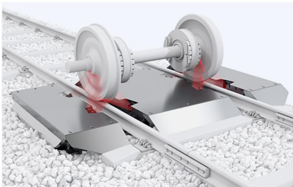
Figure 4 Ultrasound wayside NDT
