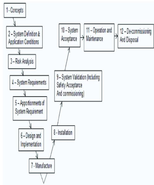
Figure 1. V diagram. Source: EN 50126.
