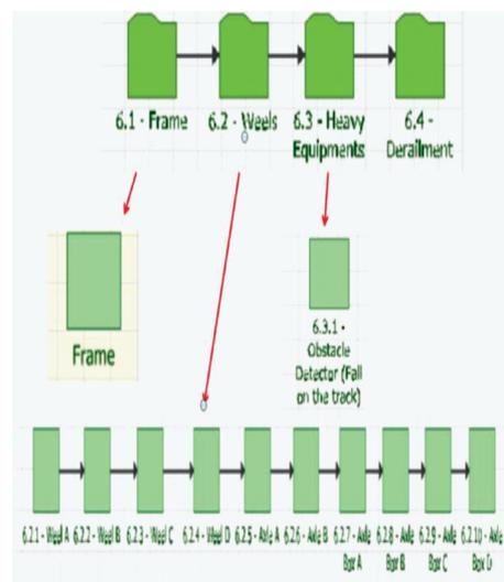
Figure 5. Bogie reliability block diagram.
