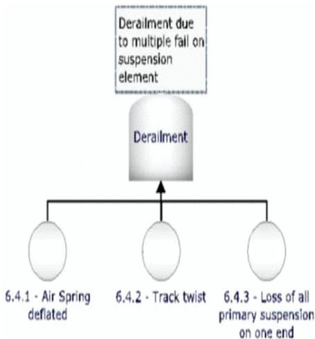
Figure 6. Fault tree analysis (derailment).
